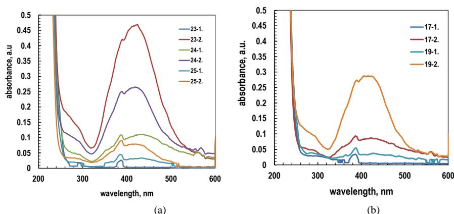
Fig. 1. UV-spectra of the Ag NPs, obtained in the presence of different initial ratio of AgNO<sub>3</sub> to Na<sub>3</sub>Cit (a) and different amount of catalyst (b)
