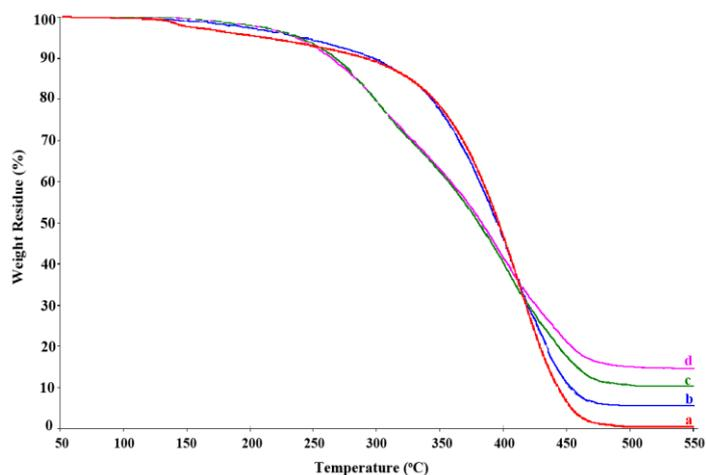
Fig. 2. TGA curves of (a) pure OBP and its nanocomposites containing (b) 0.75, (c) 1.5 and (d) 3 wt% of clay.
