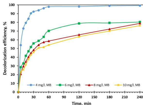
Fig. 6. Effect of MB concentration on the decolorization efficiency
