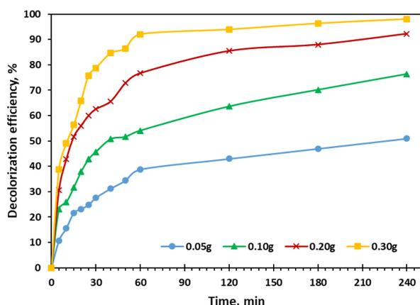
Fig. 5. Effect of nanocomposite doses on the MB removal
