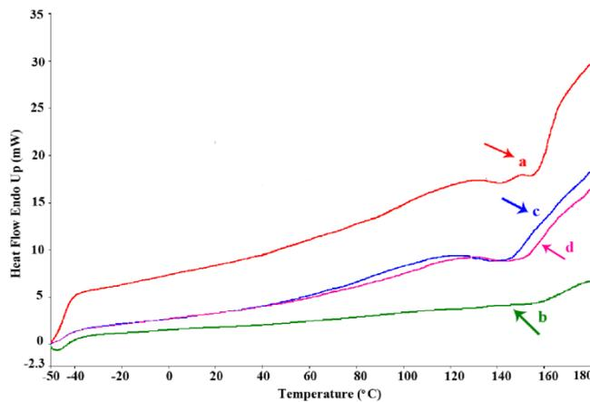
Fig. 3. DSC curves of (a) OBP and OBPCNs nanocomposites containing (b) 0.75, (c) 1.5 and (d) 3 wt% of clay
