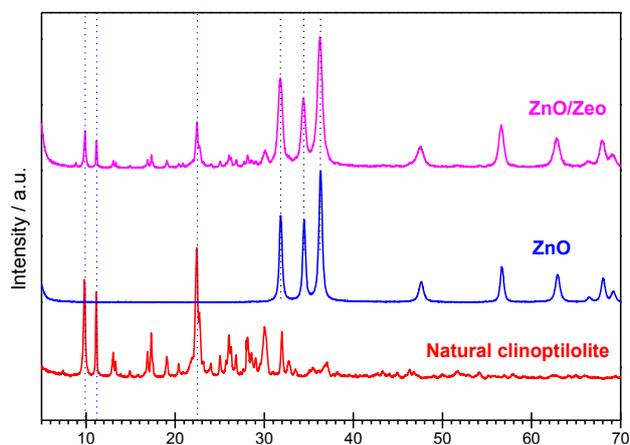
Fig. 1. XRD patterns of natural clinoptilolite, ZnO and composite ZnO/Zeo
