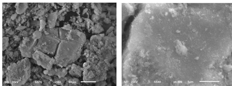
Fig. 4. SEM images of the nanocomposite ZnO/Zeo
