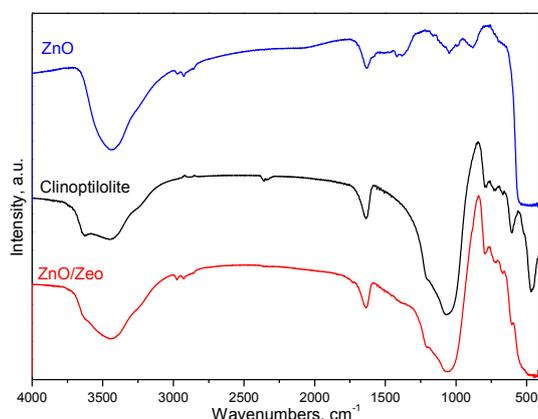
Fig. 3. Infrared spectra of ZnO, clinoptilolite and nanocomposite ZnO/Zeo
