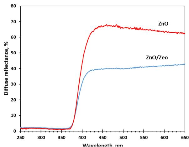
Fig. 2. UV-vis diffuse reflectance spectra of ZnO and ZnO/Zeo
