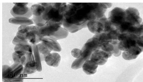
Fig. 2. TEM images of the Ag NPs, obtained in the presence of MEA (sample 23-2)
