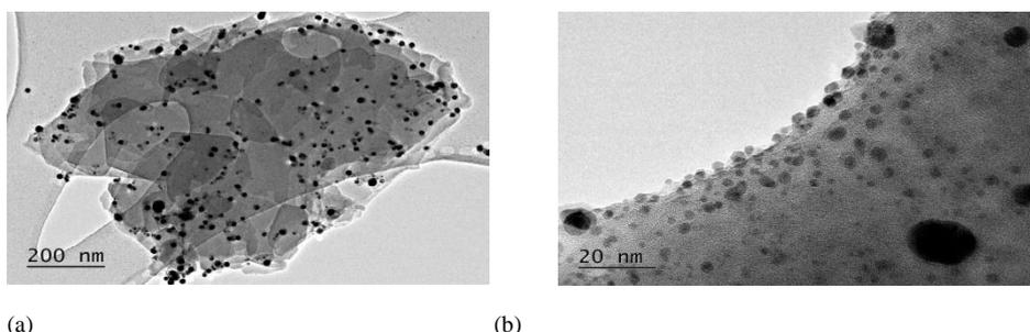
Fig. 3. TEM images of the Ag NPs-zeolite composite material, obtained by reduction of silver ions, immobilized on the zeolite, in the presence of TEA as catalyst at lower (a) and higher magnification (b)
