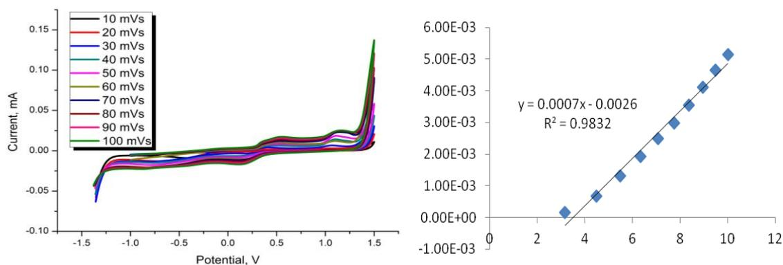
**Fig. 5.** a) PdMoAag/EupergitCM/NGCE different scan rate: 10-30-50-70-90-100  $\text{mv s}^{-1}$  in 0.05 mM  $\text{K}_2\text{Fe}(\text{CN})_6$  solution b) the plot of the peak current ( $i_p$ ) against the square root scan rates ( $v$ )<sup>1/2</sup>
