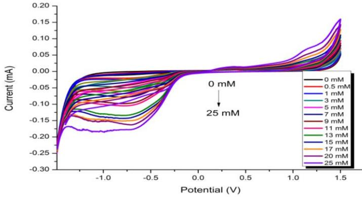
**Fig. 3.** The effect of concentration of  $\text{H}_2\text{O}_2$  on cathodic and anodic peak current in PBS (pH 7)  $50 \text{ mVs}^{-1}$ . Also, the reduction current is linearly increased with increasing  $\text{H}_2\text{O}_2$  concentration and broad peaks were obtained at higher  $\text{H}_2\text{O}_2$  concentrations. The sensor exhibited a very linear behavior in the range of 0-25 mM, after which the surface active sites were saturated.
