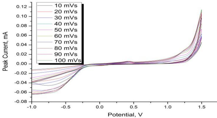
**Fig. 4. a)** PdMoAg/EupergitCM/NGCE different Scan rate: 10-30-50-70-90-100  $\text{mV s}^{-1}$  in 5 mM  $\text{H}_2\text{O}_2$  in Ar-saturated 0.1 M phosphate buffer (pH 7.5) solution **b)** The plot of the peak current ( $I_p$ ) against the square root scan rates ( $v$ )
