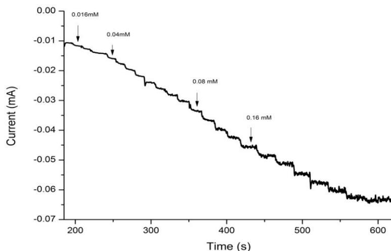
**Fig. 7.** Dependence of the CA diagrams with  $\text{H}_2\text{O}_2$  concentration in PBS buffer, pH 7,  $\nu=50 \text{ mVs}^{-1}$
