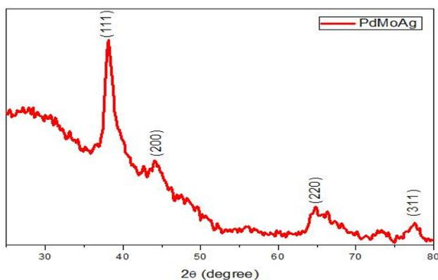
**Fig. 1.** The XRD patterns of PdMoAg catalyst
